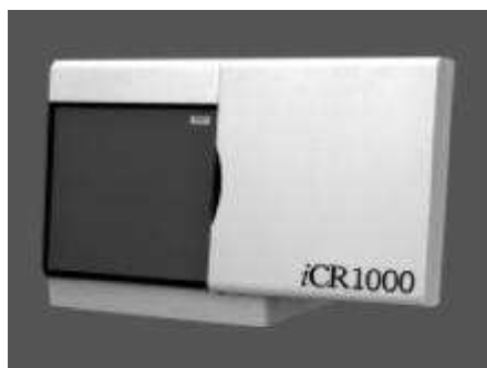
Figure 12.8 Tablet-computed radiography cassette scanner. The screen is removed from the cassette, scanned, erased, and returned to the cassette for the next exposure. The image information is sent to a computer for display and analysis. (Photo courtesy of iCRco.)
